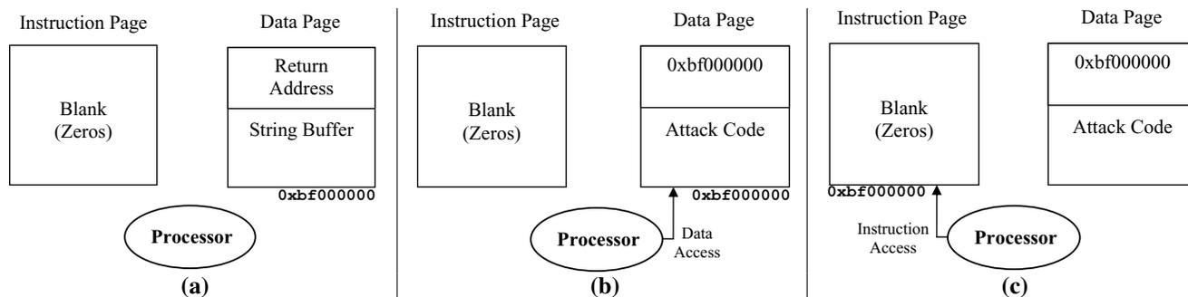
**Figure 3. (a) Before the attacker injects code (b) The injection to the data page (c) The execution attempt that gets routed to the instruction page**
