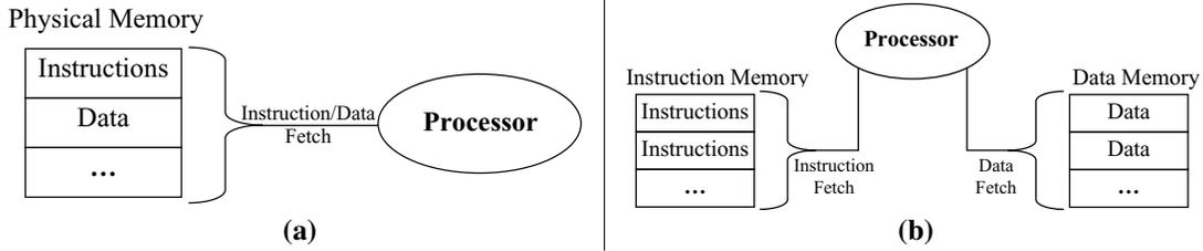
**Figure 1. (a) von Neumann architecture. (b) Harvard architecture**
