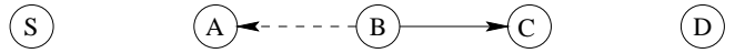
Figure 2: When B forwards a packet from S toward D through C, A can overhear B's transmission and can verify that B has attempted to pass the packet to C. The solid line represents the intended direction of the packet sent by B to C, while the dashed line indicates that A is within transmission range of B and can overhear the packet transfer.
