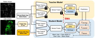
LiDAR-Radar fusion model robust to total sensor failure of one modality.
