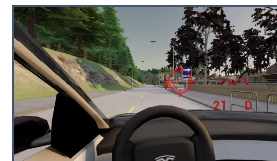
Flat-screen (spectator) view of the simulator (eye reticle at gaze point)
