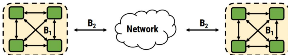
Figure 7: An example 2-level hardware topology. Solid green boxes represent GPUs. Each server (dashed yellow boxes) has 4 GPUs connected internally by links of bandwidth B_1 ; each server is connected by links of bandwidth B_2 . In real systems, B_1 > B_2 . Figure best seen in color.
